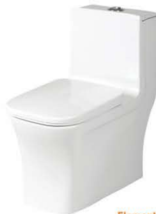
Element (OP-006) Syphonic Flush L 685 W 360 H 750 mm S-trap Central of outlet to wall 295mm
