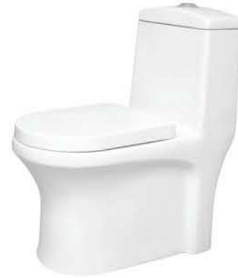
Splendor (OP-007) Syphonic Flush L 660 W 350 H 775 mm S-trap Central of outlet to wall 300mm
